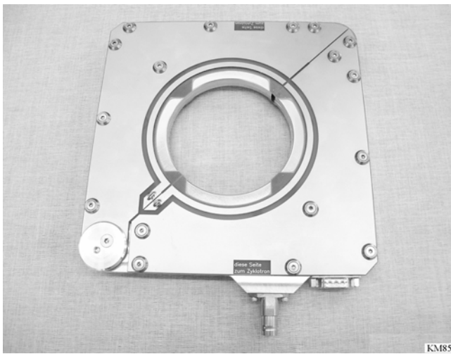
Fig. 2: halo-monitor MHH1 (to be clamped over an indentation of the beam tube, e.g. bellows) initially designed for the new PROSCAN Facility at PSI (see [5], [6]). Well visible are the high voltage electrodes of the 4 segments (the inner diameter of the device is 82 mm), which are hit directly by protons traversing the beam tube at large radii up to about 50 mm (halo).
