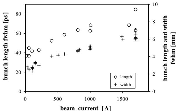
Figure 2: Phase width and radial width of beam bunches, measured at extraction from PSI Injector 2 for different beam intensities [8].
