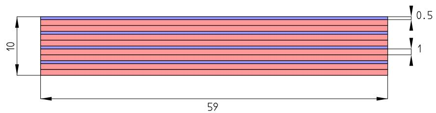
Scheme of the cross section area of a coil
